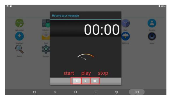
After finish recording, click **stop** menu and select **Done** to store file. The default storage path is **Internal Memory/Android/data/com.android.soundrecorder/files/Download**
