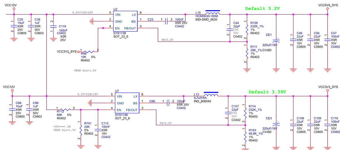
$$V_{out} = 0.6 * (1 + R_{114} / R_{153})$$
